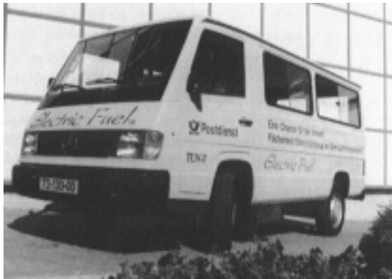
Figure 2: German Postal Vehicle with Zinc-Air Battery [2]
