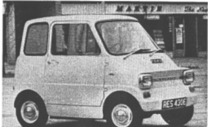
FIG. 1 Comuta electric car developed by Ford of Britain is very limited in range, 37.5 miles at a steady 25 mph being a simple performance, and the top speed is 40 mph. This 1550-lb vehicle, 384 lb of which is battery weight, is able to transport two adults and two children.
