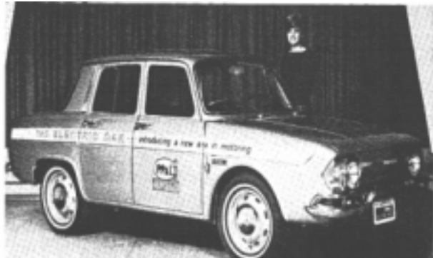
FIG 3 MARS 11 electric car developed by Electric Fuel Propulsion uses tripolar, lead-cobalt cell design in four 30V, 290-amp-hr batteries to propel its 4260-lb weight. Regenerative braking is also used to help attain a single-charge range of 70-120 miles, Top speed is 60 mph.
