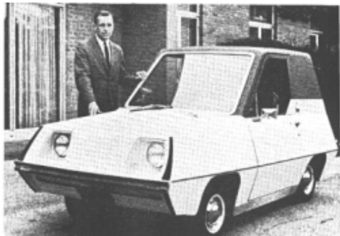
FIG. 2 Delta electric car developed by General Electric uses the hybrid lead-acid, nickel cadmium battery concept to attain a top speed of 55 mph and a range of 100-120 miles at a steady 30 mph. The vehicle weighs 2300 lb and can carry two adults plus two or three children.
